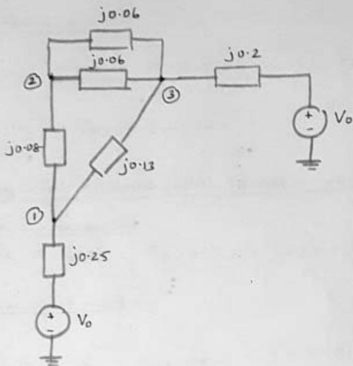
The positive sequence network of a three-bus power system is shown in fig. For a symmetrical 3 $\phi$  to ground fault with  $Z_f = j0.1$  p.u. Find the fault currents for faults at buses 1, 2 and 3. For fault at bus 1, find all bus voltages and line currents. Assume  $V_0^a = 1 + j0$ .
