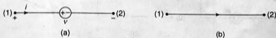
**Fig. 3.4** Voltage source and its oriented graph.
