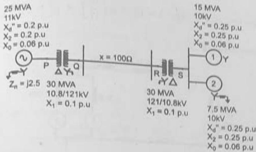
subtransient reactance. Draw the zero sequence network of the system assuming zero sequence reactances of generator and motor as 0.06 p.u. Current limiting reactors of  $2.5\Omega$  each are connected in the neutral of generator and motor no. 2. The zero sequence reactance of transmission is  $100\Omega$ .
