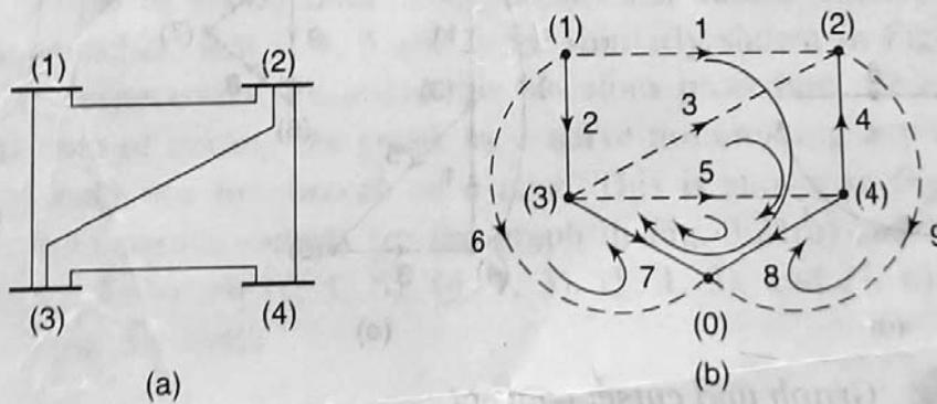
**Fig. 3.18** Transmission, network, graph tree and co-tree
