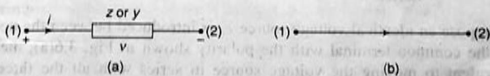
**Fig. 3.5** Generalized circuit element and its oriented graph.
