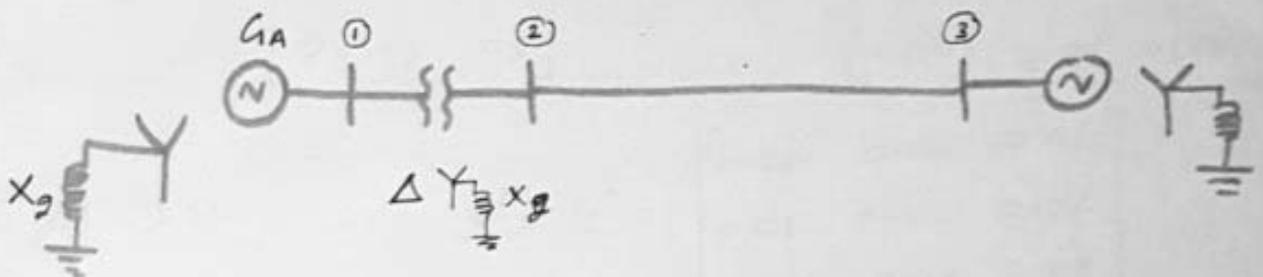
The fig. shows the one-line diagram of power system. Impedance data are as follows.
