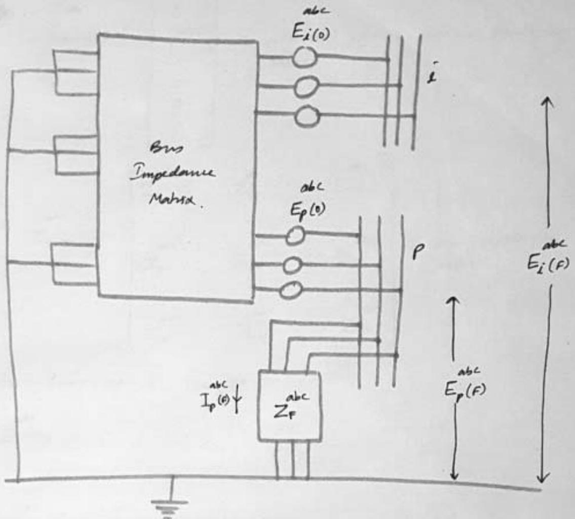
The representation of the system with a fault at bus 'p' is shown in fig. In this representation, derived by means of Thevenin's theorem, the internal impedance is represented by the bus impedance matrix including machine reactance and the open circuited voltage is represented by the bus voltage prior to the fault.
