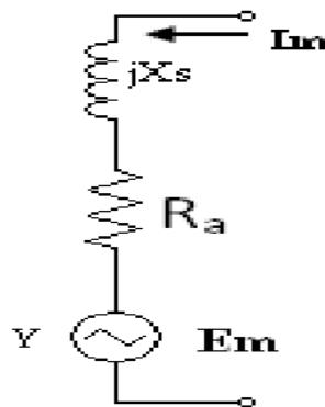
1Φ equivalent circuit of synchronous motor
