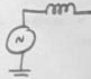
④ If the resistances of the transmission lines are smaller than the reactances by a factor of six or more, the resistances are neglected. For high voltage systems  $X/R \gg 6$  and hence  $R$  is neglected.
