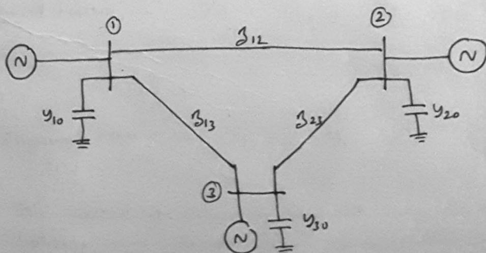
The total capacitance susceptances at the buses are represented by  $Y_{10}$ ,  $Y_{20}$ , and  $Y_{30}$ . Applying KCL at each bus, we get
