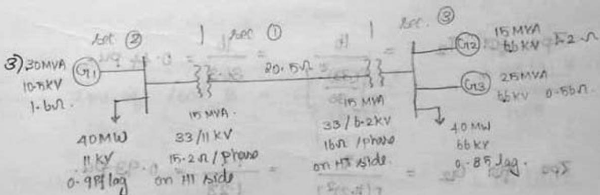
Obtain the per unit impedance diagram of the power system shown in figure. Assume a base of 30 MVA, 33 kV on the transmission line.
