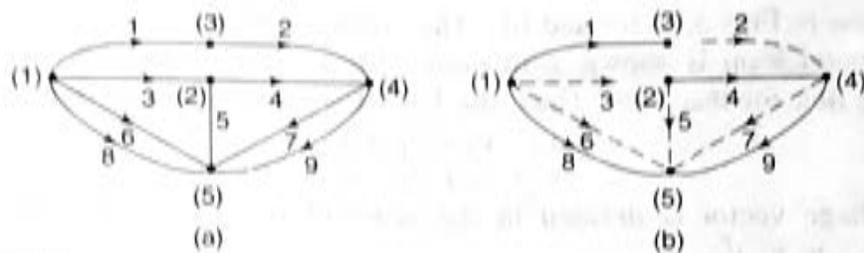
**Fig. 3.15** Graph, tree (solid) and the links (dotted).
